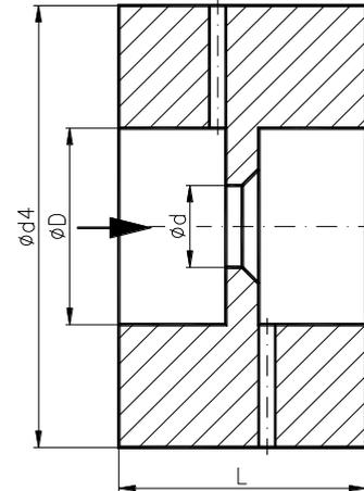
according to the relevant standards (ISO 5167, ASME MFC-3M etc.). The plate type is chosen based on the specific process conditions. The orifice plate edge is typically manufactured from a wear-resistant material like stainless steel. The material of the carrier ring can be equivalent to the pipe material.
